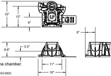
Pro4 LP® Endcaps can be installed at either end of the chamber.
