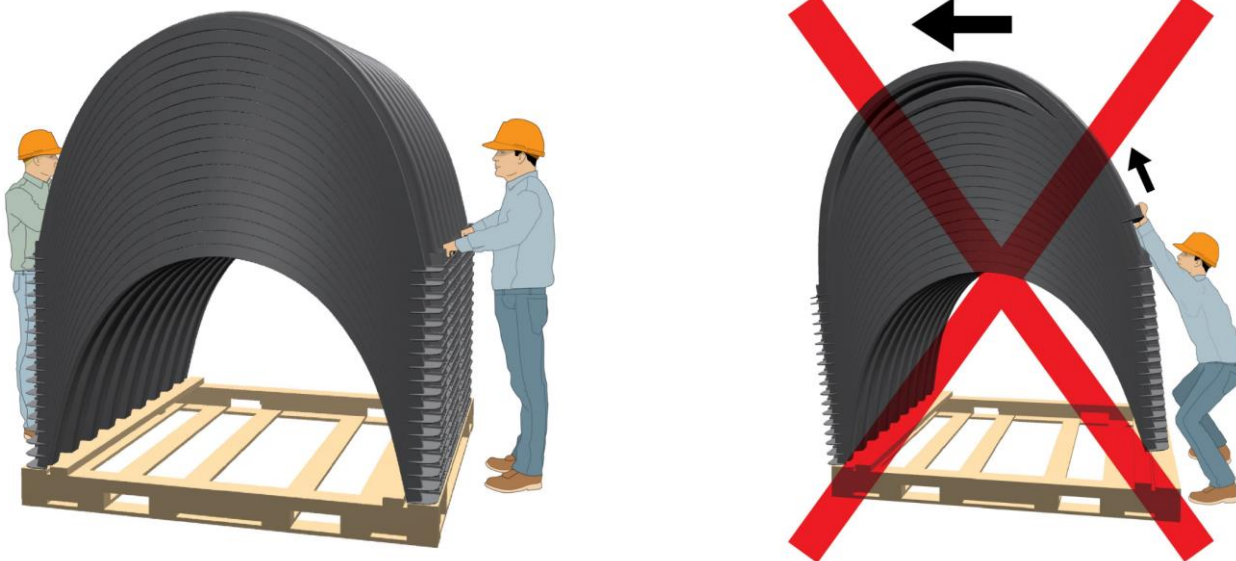
Figure 4 - Chamber Unloading from Pallets
